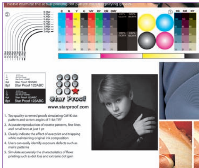
Characterisation charts assist in initial press fingerprints and ongoing press colour management
